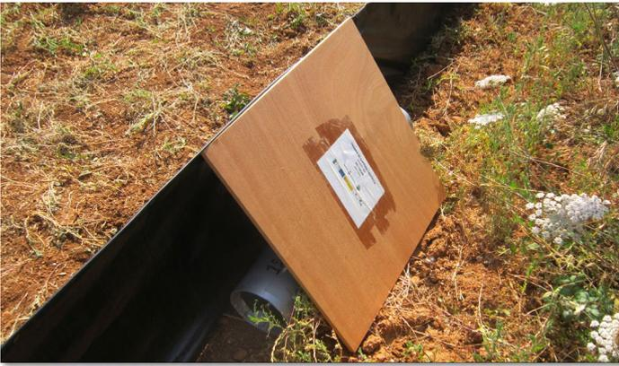
Fig. 40. A PVC double funnel trap for snakes covered with plywood panels.
