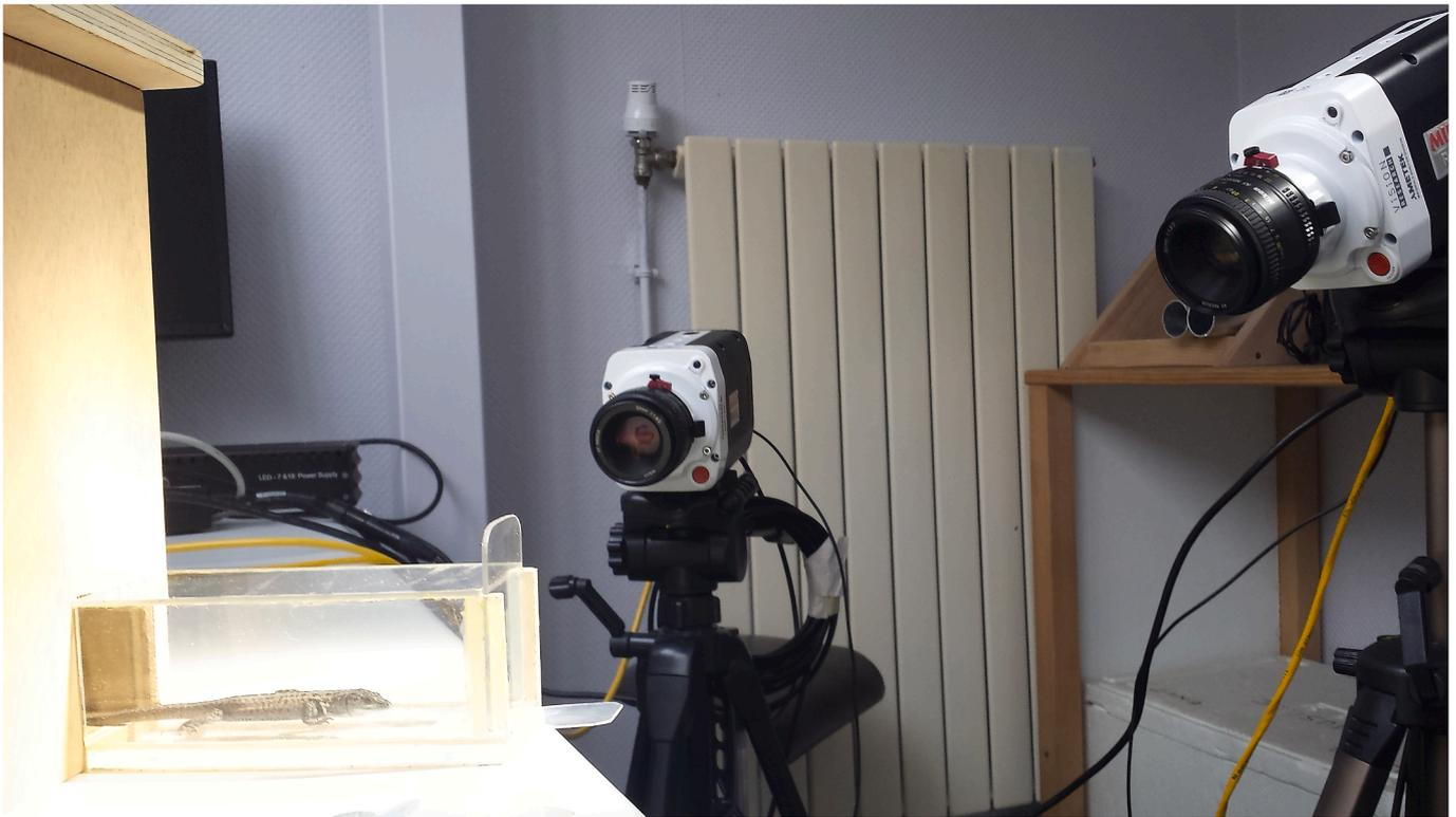
**Fig. 1.** Picture of the experimental set-up showing the two high-speed cameras pointing to the end of the tunnel where the prey is positioned. Note the relative position of the cameras which are oriented to form an acute angle allowing to optimize camera calibration and to enhance the accuracy of the three-dimensional tracking.
